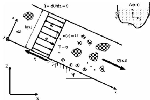
**Fig. 1** Avalanche flow is described by two scalar fields  $A(x,t)$  and  $Q(x,t)$ . The first field  $A(x,t)$  represents the cross sectional flow area at  $x$  and time  $t$  and the second field  $Q(x,t)$  gives the average snow discharge along the mountain profile (Bartelt et al., 1999). A Voellmy-fluid flow law is applied that assumes no shear strain-rates in the avalanche flow plug.
