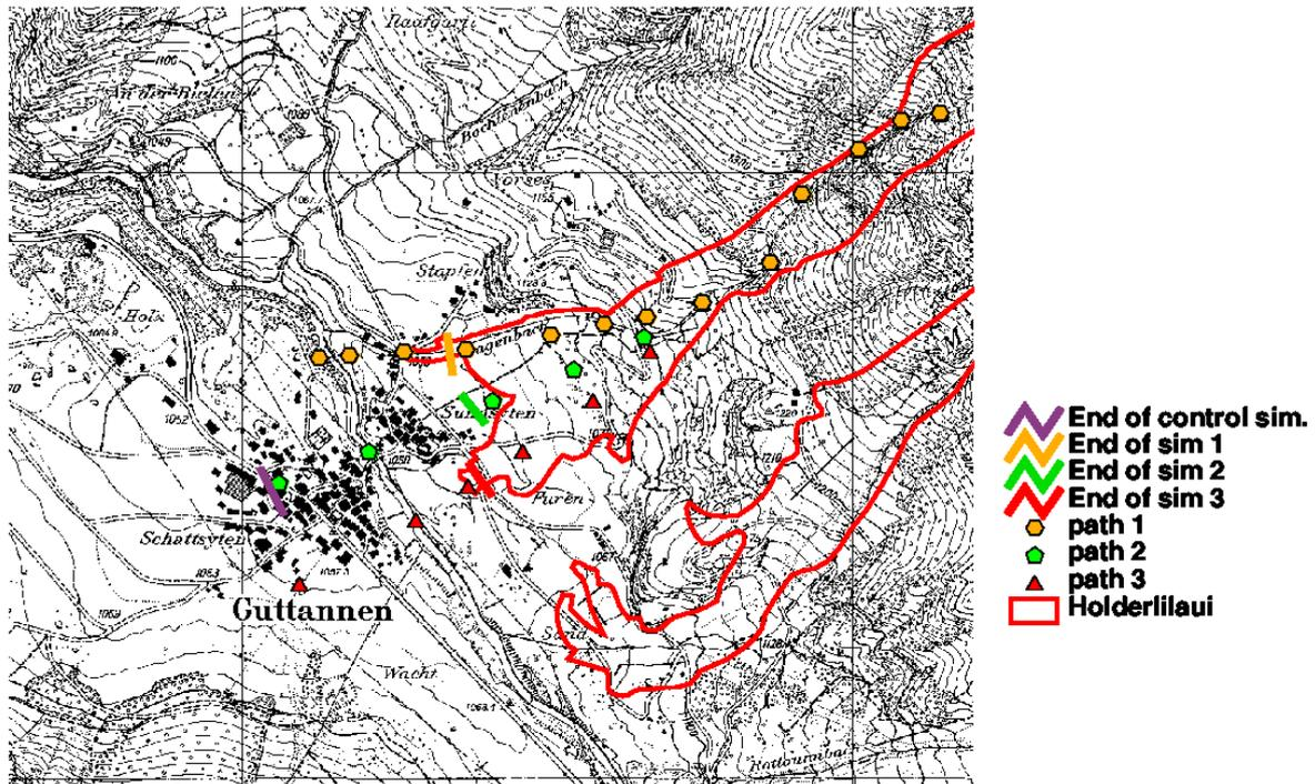
**Fig. 6** Map showing the three paths in the runout zone of Holderlilau. The stopping points of the control simulation and the split simulations are marked.
