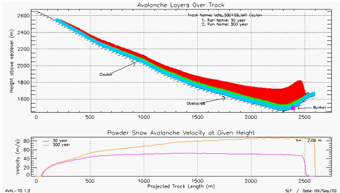
**Fig. 7 Upper window: Snowcover (blue), saltation layer (green) and suspension layer (red) with three points of interest (couloir, obstacles and bunker). Lower window: Maximum velocities at a height 2m above the ground for 30 and 300 year avalanche.**
