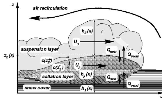
Fig. 2 Schematic view of the structure of a powder snow avalanche according to Norem (1995). Some quantities relevant to the model are also indicated. Subscripts 1, 2, 3 on field variables generally refer to the snow cover, saltation layer and suspension layer, respectively (Issler 1998).
