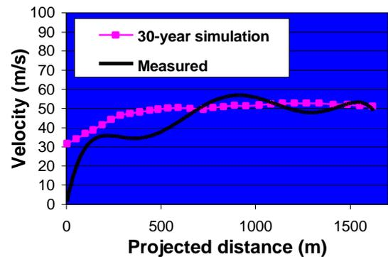
**Fig. 8 Measured and simulated velocities along the Vallée de la Sionne avalanche track.**
