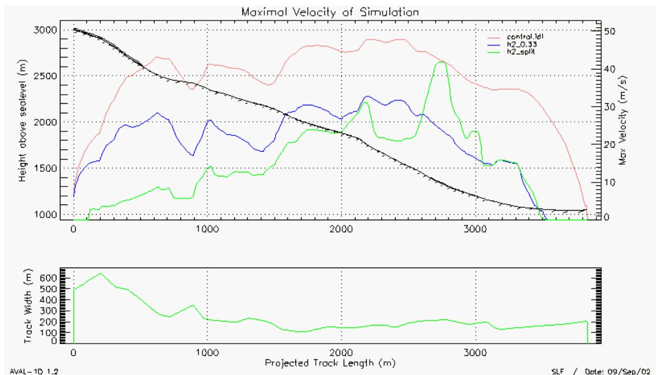
**Fig. 5** A comparison between maximum velocities of control simulation (*control.idl*), a run with reduced (33%) release mass (*h2\_0.33*) and the split simulation (*h2\_split*, 15% from point 1160m a.s.l.).
